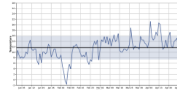
(a) Statistical process charts rely on comparison to an expected value, and so deviations from that value, not from zero, are important
